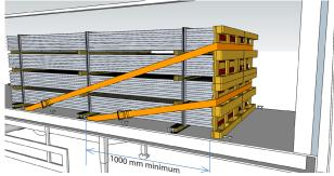
\*Load restraint straps removed for image clarity.
